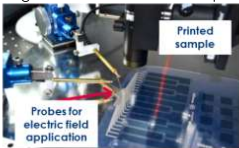
Figure 8. Direct probes poling process.
