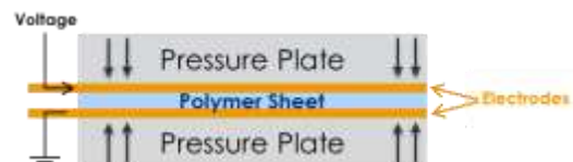
Figure 9. Contact poling process.
